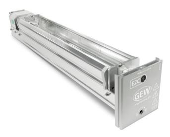
E2C cassettes are designed and manufactured for the harshest environments, with optically tuned reflectors to maximise the lamps' curing effect. To maintain the long-term operation of the UV system the cassettes should be serviced regularly (every two years). The service can increase the output of the cassette by up to 70%.
